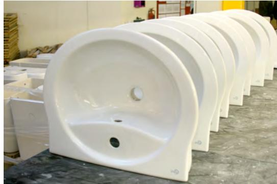
Completed product after glazing and kiln firing
