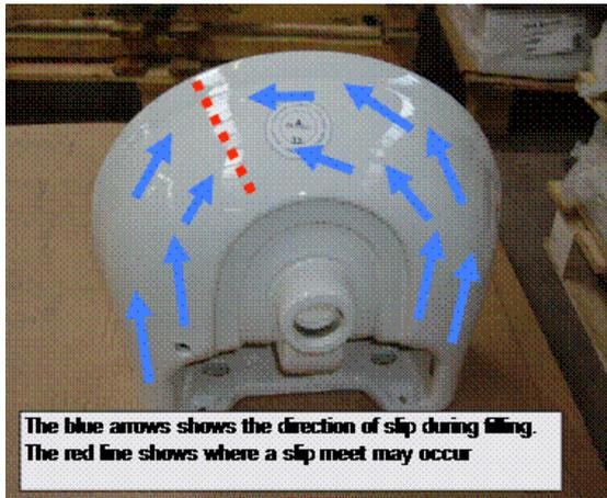
'Slip meet' is a term used to describe a fault in the pot and happens as the mould is filled with the slip. Imagine the inside of a basin mould filling with clay from the bottom upwards, the slip will firstly fill the base of the mould and then travel upwards. The 'slip meet' will be located at the point where the last bit of air leaves the mould and the slip meets together.
